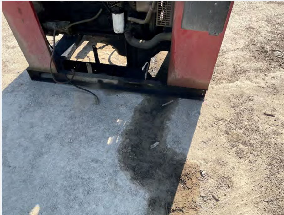
49. Soil staining beneath abandoned diesel motor located near the irrigation supply groundwater wells.
